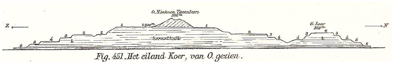
Figure VII.1.9. Historic S-N cross-section through Kur Island (West of Kai islands), showing six Quaternary reef terraces up to 300m elevation, and core of dipping mica schist and ?Miocene micaceous sandstones (Verbeek 1908).
