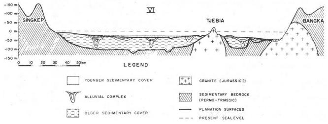
Figure XI.4.2. NW-SE cross-section from Singkep- Cebia to Bangka island, showing steeply dipping Permo-Triassic metasediments, intruded by Late Triassic granitoids, overlain by thin Miocene sediments and a Pleistocene Alluvial Complex of 30-45m deep tin-bearing incised valleys and very thin Late Quaternary sediment cover (Aleva, 1973).
