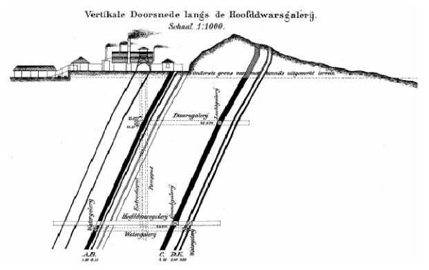
Figure XI.3.2. W-E cross-section across Pengaron coal mine in Eocene coal, Barito Basin, SE Kalimantan (Hooze, 1893). This government-operated mine was the first and one of very few underground coal mines in Indonesia.
