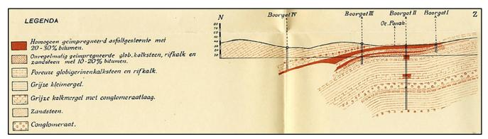
Figure XI.1.4. Cross-section showing near-surface asphalt impregnation in Miocene rocks in Panah asphalt terrain, Buton (Hetzel 1936).
