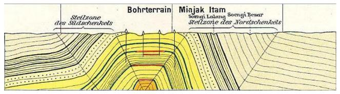
Figure XI.1.6. Example of oil-bearing anticlinal structure: SW-NE cross-section across part of the Kampung Minyak oilfield, S Sumatra (Tobler 1906).
