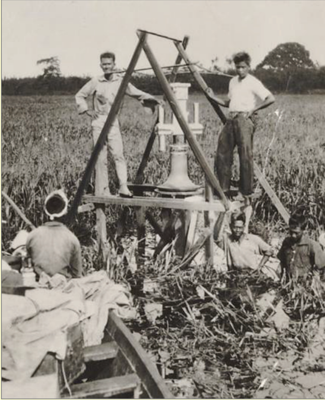
Fig. XIV.153. A torsion balance gravity survey crew in a swamp in Sumatra (probably a BPM crew in the late 1930s) (Coll. KITLV 140177). The instrument is probably a German-built Askania Z-40 Z-beam torsion balance, which would require 40 minutes to complete one station measurement. A gravity survey crew working day and night could set up and measure about eight stations per day.
