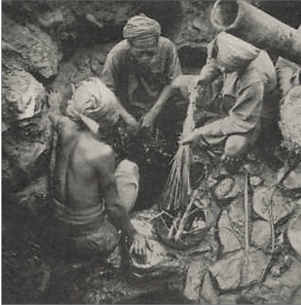
Fig. XIV.3. Collecting oil from a natural oil seep on the Ledok anticline, NE Java (Witkamp, 1917). A bundle of rice straw is dipped into the well, and then squeezed out into a bowl made from palm leaf.
